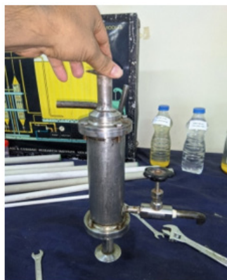
Figure 5: Membrane module made up of SS316.
