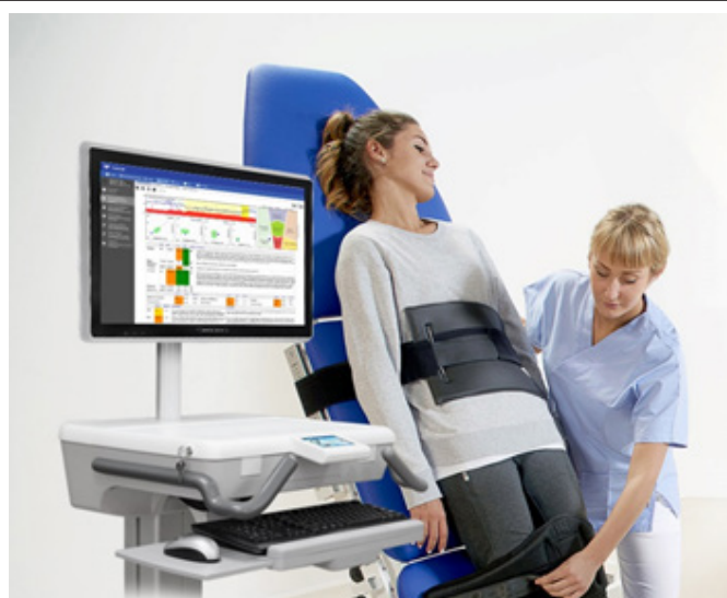
Figure 1: This is an image of the VitalScan-ANS System developed by Medeia Inc. performing the tilt table test. The VitalScan-ANS System is portable, easy-to-use, and non-invasive.
